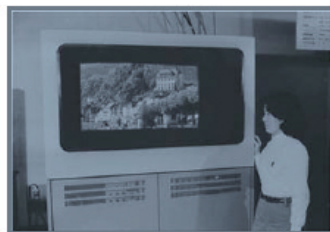
Wide display with 1,125 scanning lines (combining three cathode-ray tubes)
